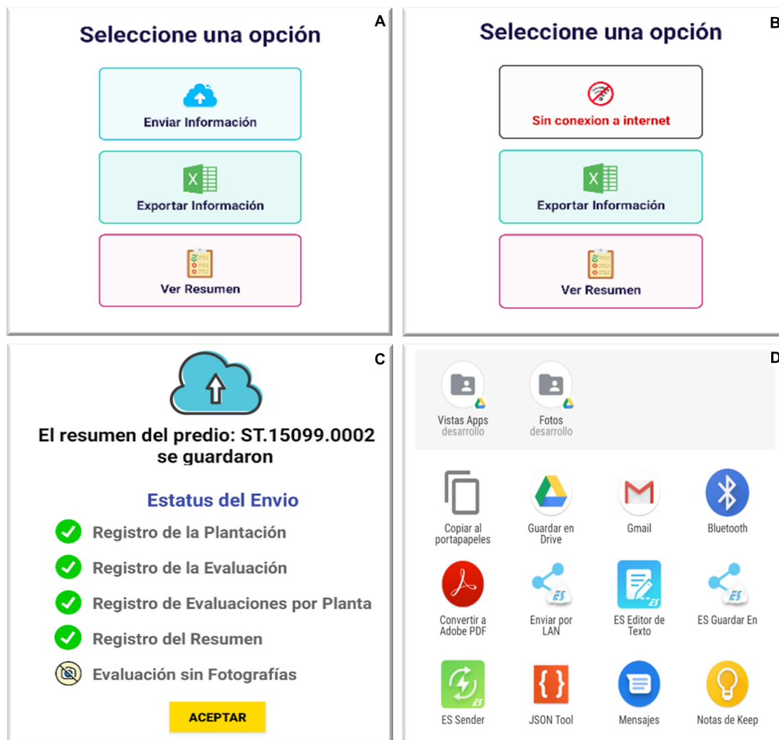
Figure 7. Interface of the App-ExploraCítricos v2.0 for the management of assessment records of citrus farms. A. Log management options include 'Sending' to the web repository using Wi-Fi or mobile plan; 'Export' in MS Excel; and see 'Comprehensive Reports' of an assessment at 'Farm' level. B. Automatic view indicating that only the 'Export' and 'Report' options are functional due to local lack connectivity. C. Example of a report on the successful sending of a record/farm to the web repository. List of core modules successfully submitted and a ID assigned to the farm. In case of failures or missing data per module, an error icon indicates it. D. View of options to export data from MS Excel for each farm. They include mail, bluetooth, drive, and social networks like MSN or others.
